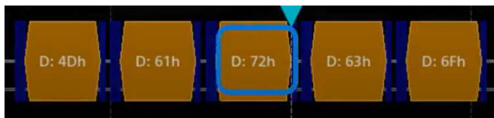
Figure 13-13: Trigger on Type= Tx, Data =0x72 and Position=3
