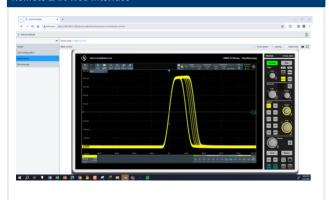
Interact with Rohde & Schwarz scopes using the built-in web browser. The front panel makes has buttons and dials in addition to the setting dialog. Make and download screen images with a mouse click.
