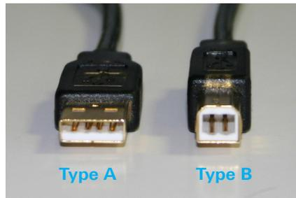
Fig. 1.1: USB type A and type B
