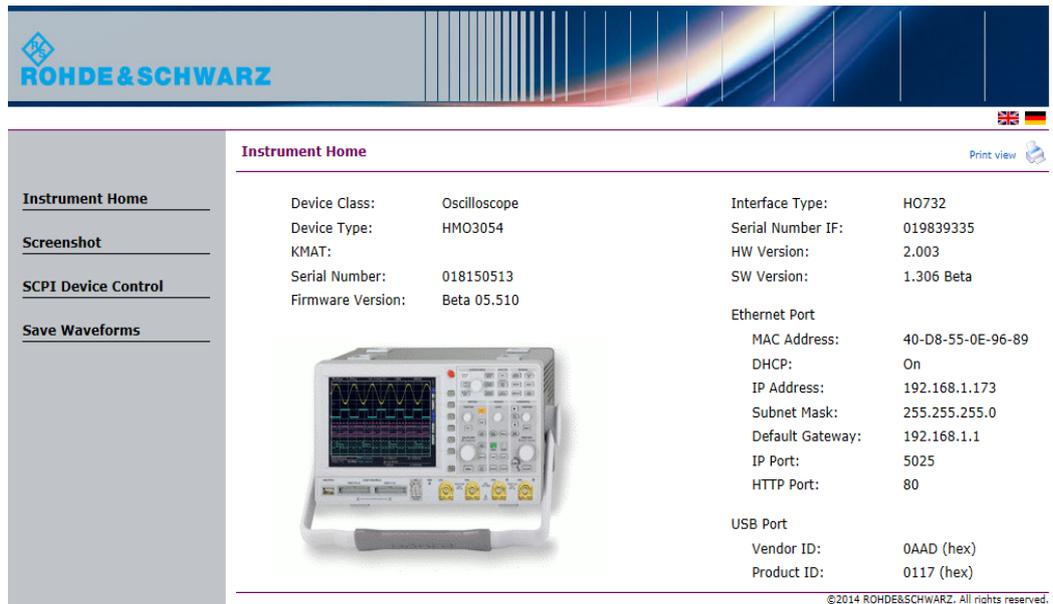
Fig. 3.2: Display of the device and Ethernet information
