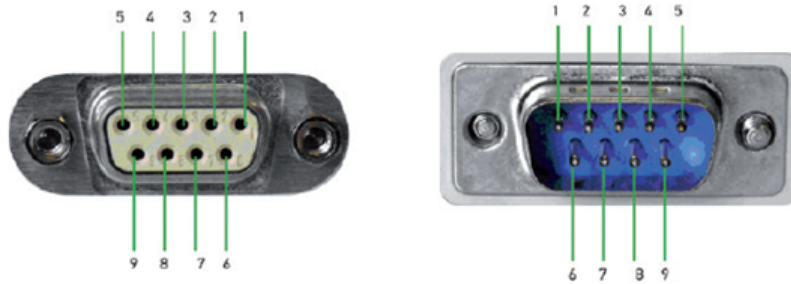
Figure B-2: RS232 Pin Assignment
