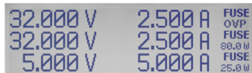
Figure 4-6: Overvoltage protection (example R&S HMP2030)
