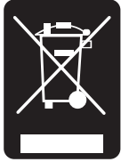
Fig. 1.4: Product labeling in accordance with EN 50419
