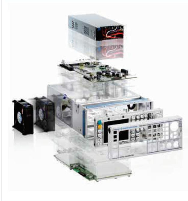
A minimum of modules in the R&S SMC100A means high reliability and easy servicing.
