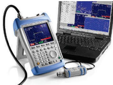
The R&S®FSH can be remotely controlled via the USB or LAN interface and integrated into user-specific programs.
