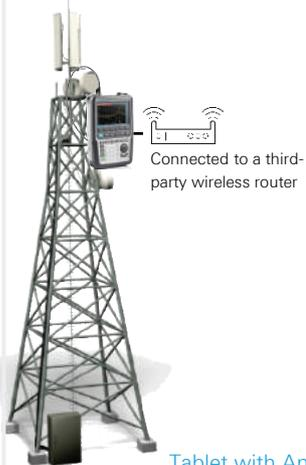
Tablet with Android/iOS app to remotely control the analyzer.
