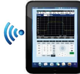
Wired/wireless\* remote control with R&S®InstrumentView PC software
