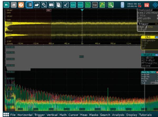
R&S®RTE oscilloscopes come with built-in spectrum analysis for up to four signals in parallel. Results can be correlated in the time and frequency domain. Analysis functions such as spectrogram (with R&S®RTE-K18 option), mask test and peak list are available.
