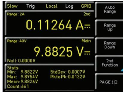
Simultaneous display of three measurements, including DCI and ACI at the same time.
