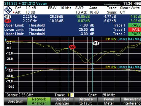
For cable loss and antenna testing and characterization as well as distance to fault measurements.
