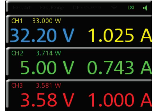
The different operating conditions are marked by colors: constant voltage operation is indicated in green, constant current operation in red, inactive channels are shown in yellow, blue indicates that the channel is in setting mode.
