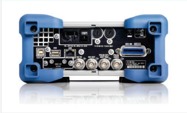
Integrate into current test setup without having to alter your USB, Ethernet or GPIB connectivity interface.
