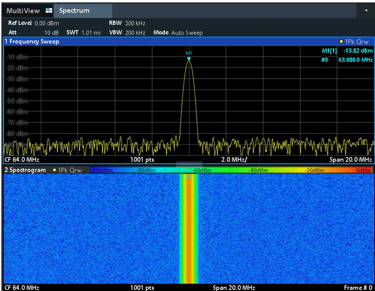
Figure 7-4: Spectrogram of the calibration signal
