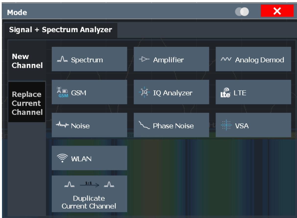
*Figure 7-5: Adding a new measurement channel*
