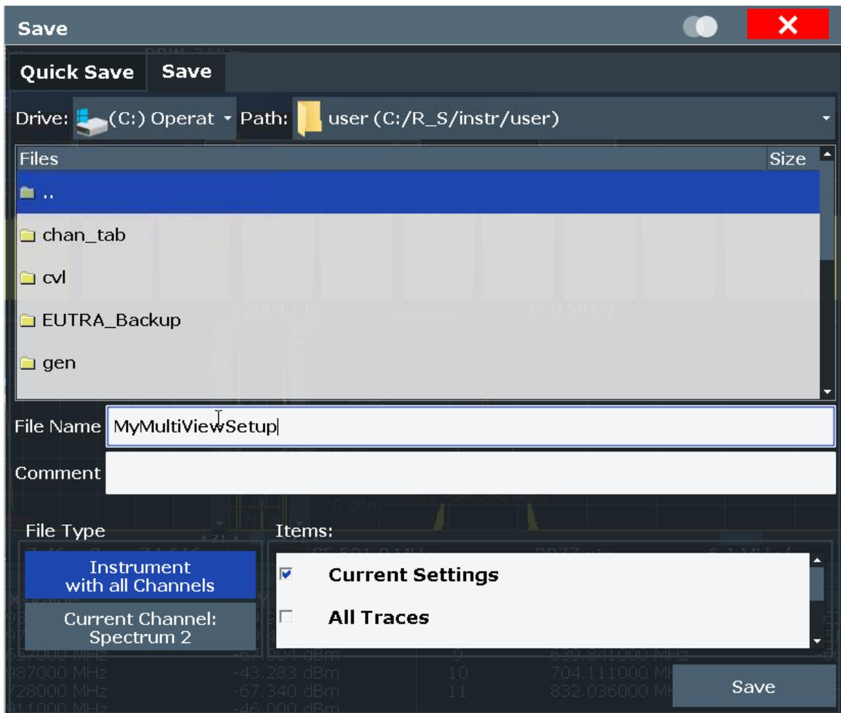
**Figure 7-17: Saving the instrument settings to a file**
