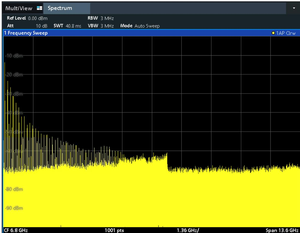
**Figure 7-1: Calibration signal as RF input**
