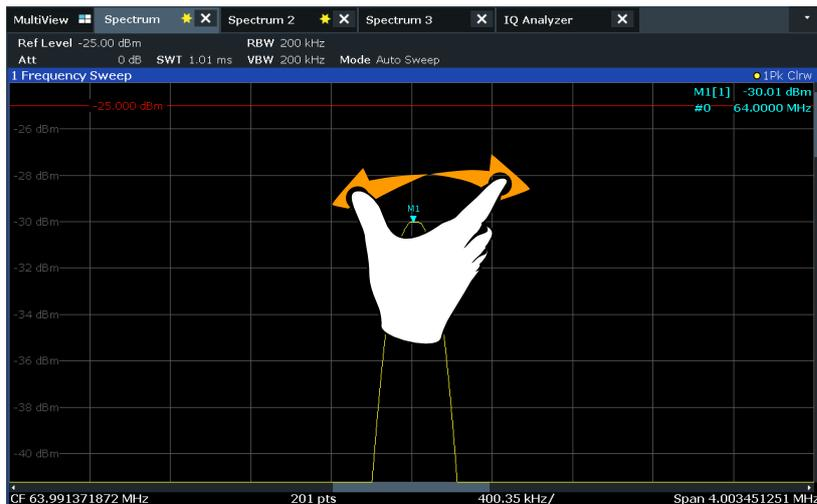
The area around the marker is enlarged in the result display.
