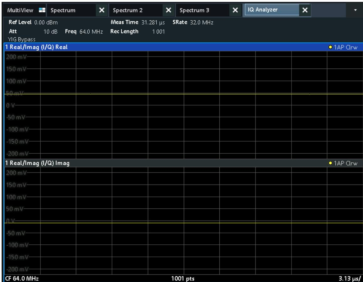
**Figure 7-8: Inserting a Real/Imag diagram for I/Q analysis**
