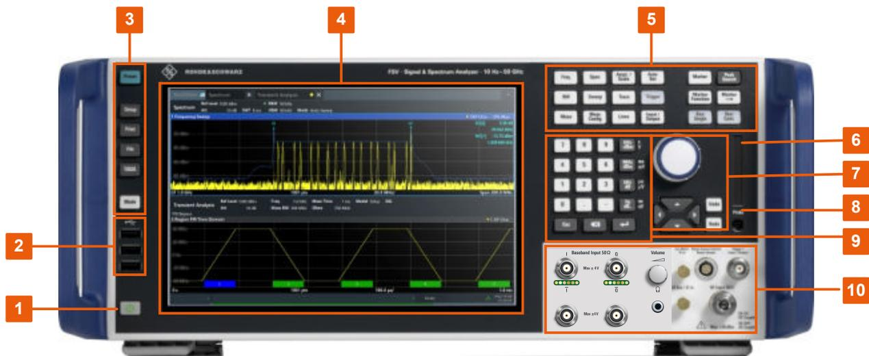
Figure 6-1: Front panel view of R&S FSV/A
