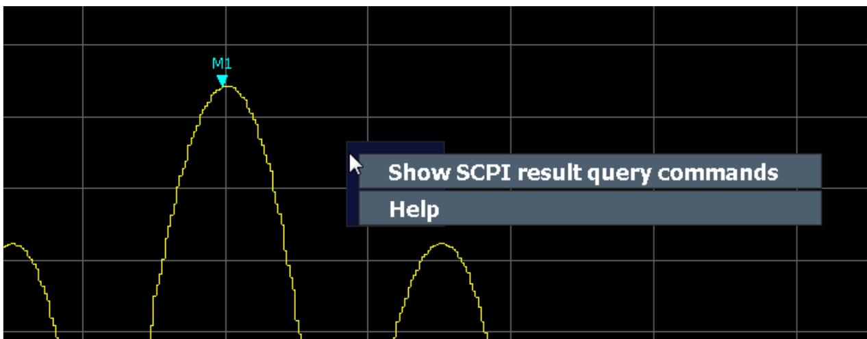
**Figure 8-1: Context menu for a result display with SCPI Recorder functions**
