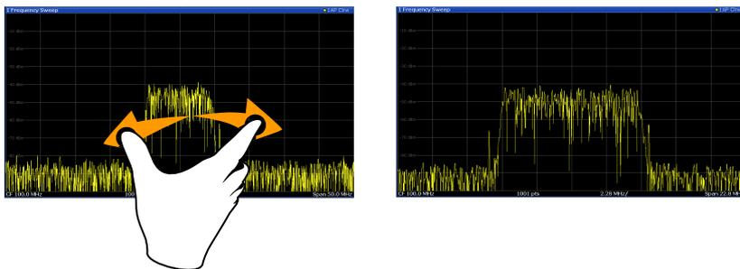
**Figure 8-6: Spreading**
