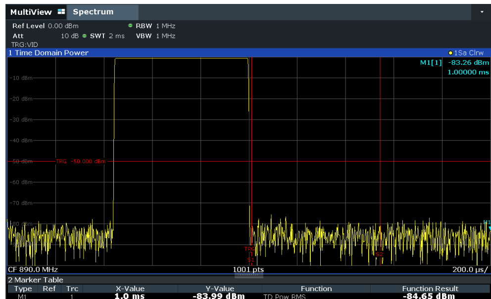
Figure 7-19: Measurement of the signal-to-noise ratio of a GSM burst signal in zero span
