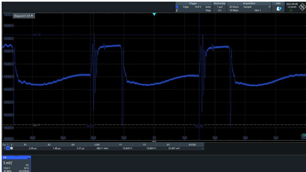
Figure 22 Ripple Voltage @ Full Load
