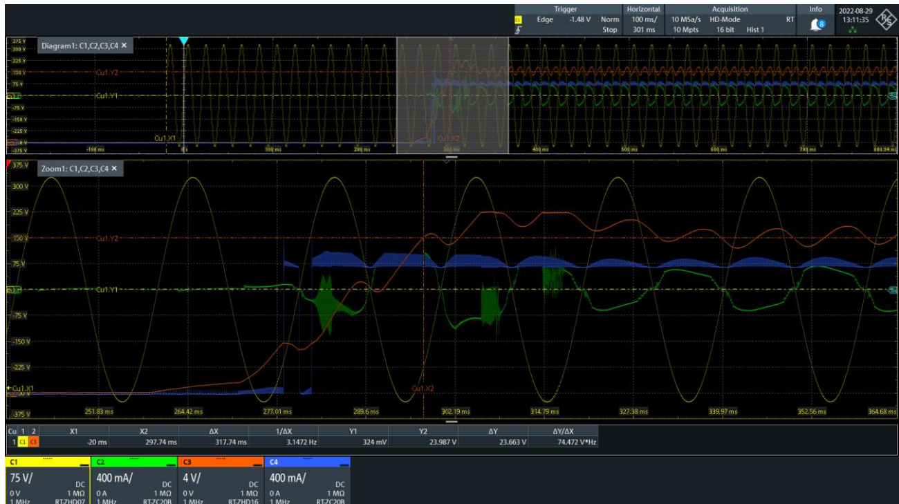
Figure 30 Turn-on Delay Measurement
