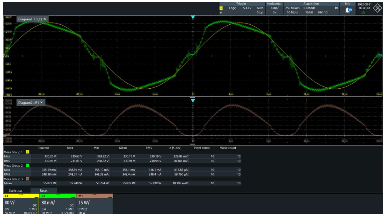
Figure 9 Measured Voltage, Current and Power at Input Terminals
