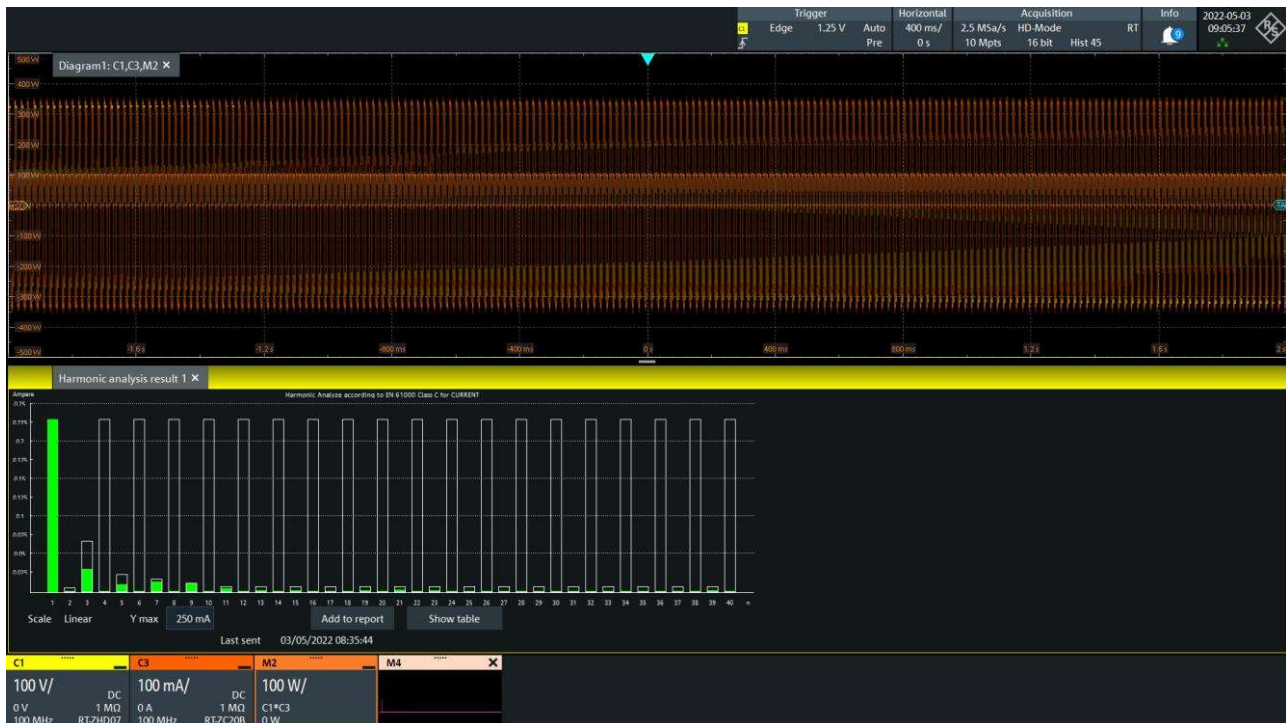
Figure 13 Current Harmonic Measurement Bar View
