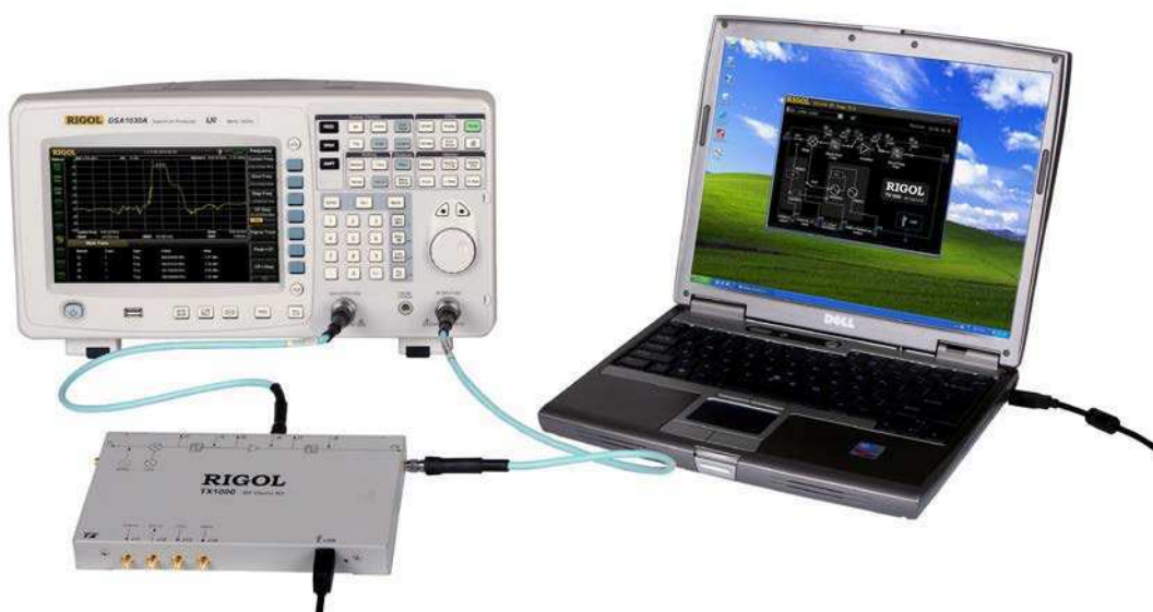
Figure 7 Test the Band-pass Filter Characteristics
