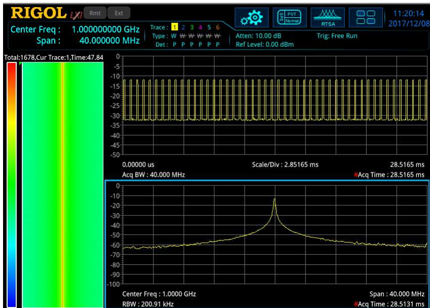
Figure 3-7 PvT Spectrogram View
