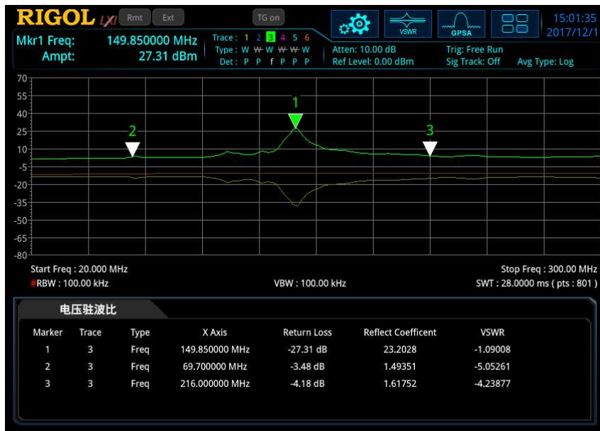
Figure 2-13 VSWR Measurement Interface
