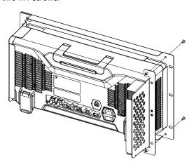
4. Get encased in the cabinet: Mount the assembled instrument and rack into a standard 19-inch cabinet by using six M6 screws and six M6 square nuts.
