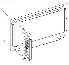
2. Place the instrument: Place the instrument into the frame set up by the front plate and the left plate.
