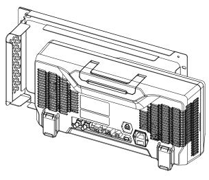
3. Install the right plate: Attach the right plate to the right edge of the front plate, then fasten them with two M4 screws.
