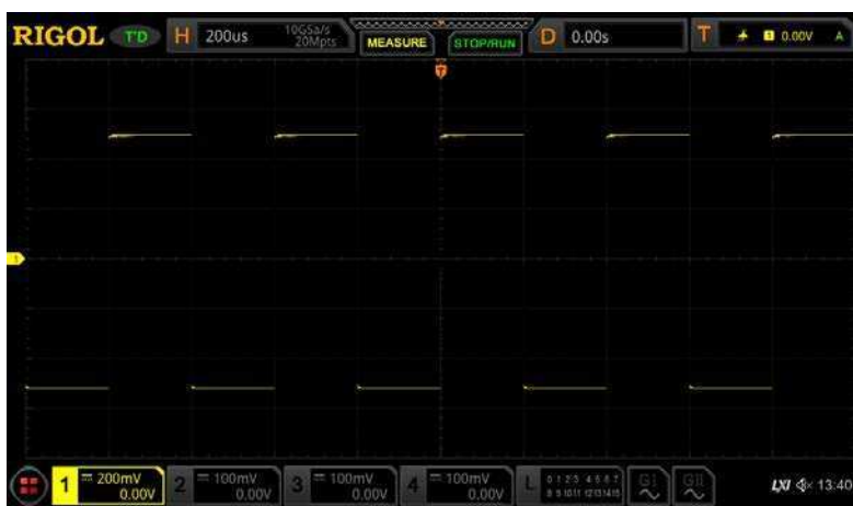
Figure 4-3 Waveforms after 128 Times of Averaging
