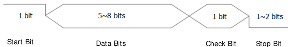
Figure 5-13 Schematic Diagram of RS232 Protocol
