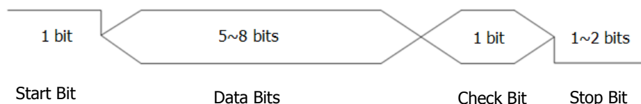
Figure 5-13 Schematic Diagram of RS232 Protocol
