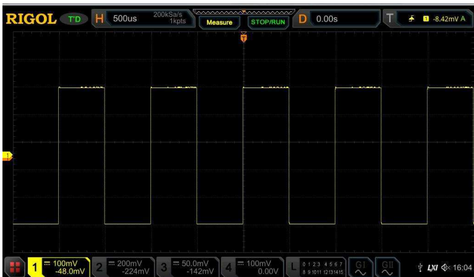
Figure 4-3 Waveforms after 128 Times of Averaging
