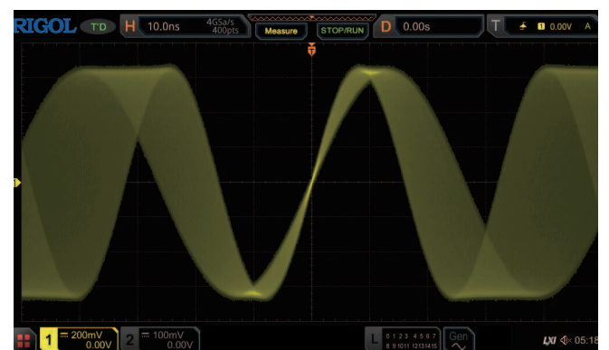
Changes of each frame of waveforms of the sweep signal can be clearly observed in the highly refresh mode.
