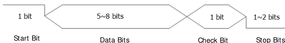
Figure 5-2 RS232 Bus Frame Format
