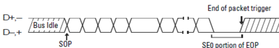
Figure 5-8 USB Data Transmission Protocol
