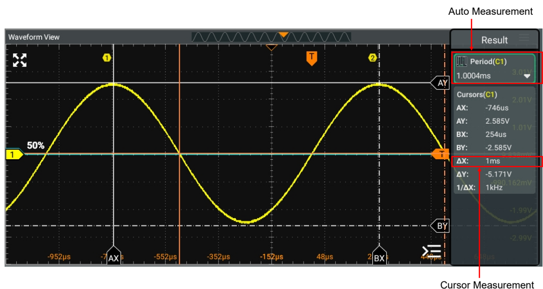
Figure 10.9 Manual Cursor Measurement Example
