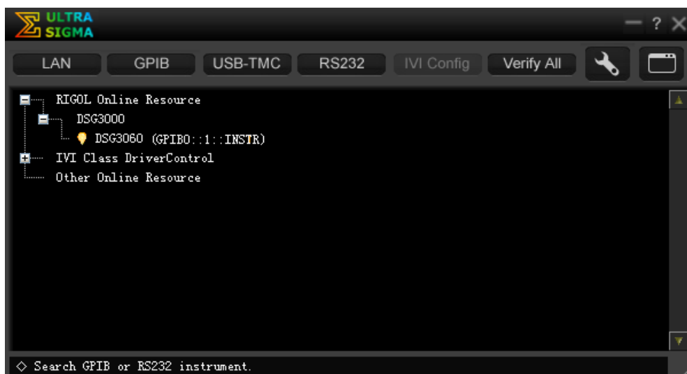
Figure 3-8 View the GPIB resource
