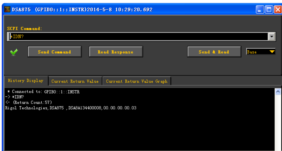
Figure 3-9 Write and Read Commands via GPIB
