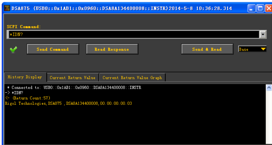
Figure 3-2 Write and Read Commands via USB
