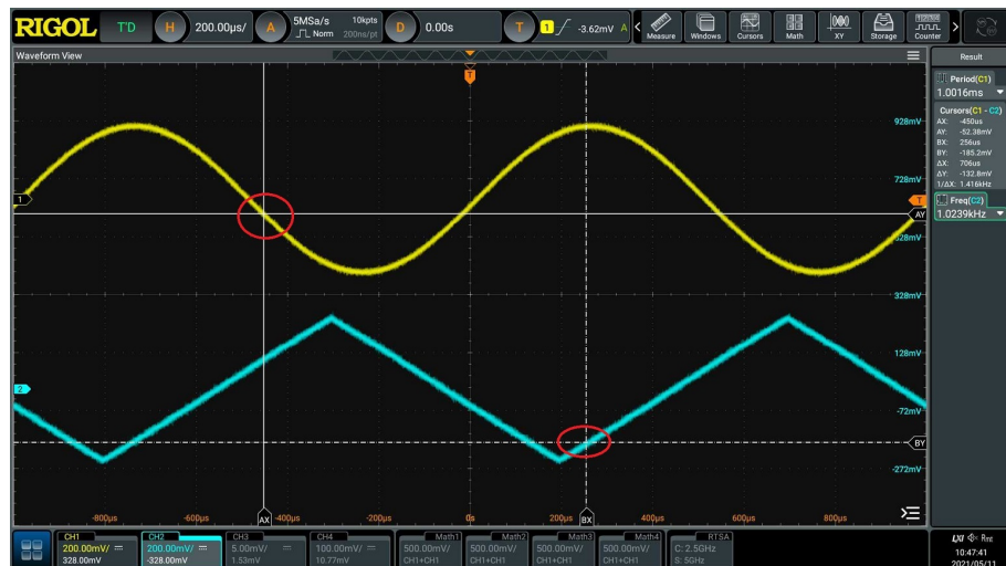
Figure 10.14 Track Measurement (after Horizontal Expansion)
