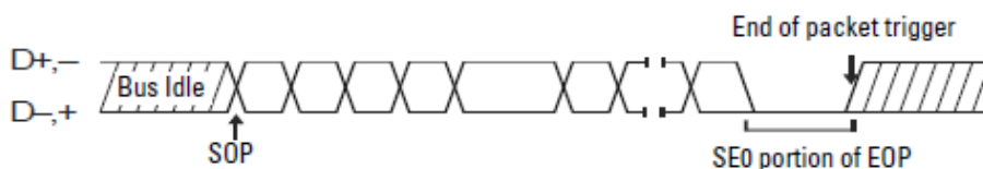
Figure 5-9 USB Data Transmission Protocol
