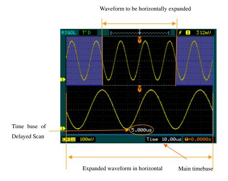
Figure 2-39: Delayed Scan window
