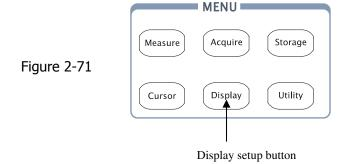
Press the Display button to pop up the menu for the settings of the display system.
