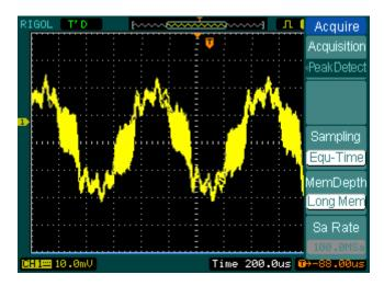
Figure 2-70: Signal with Peak Detect Acquisition
