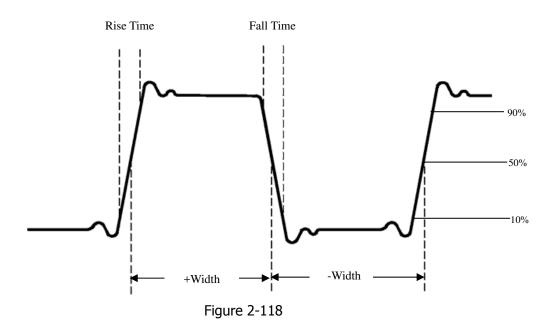
**Rise Time:** Time that the leading edge of the first pulse in the waveform takes to rise from 10% to 90% of its amplitude.
