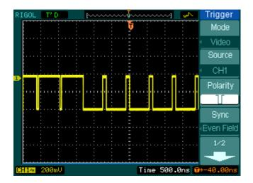
Figure 2-49: Video Trigger: Field Synchronization
