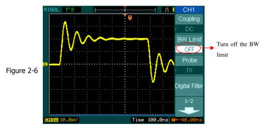
Press CH1→BW Limit→ON, to set up bandwidth limit to "ON" status. It will reject the frequency component higher than 20MHz.
