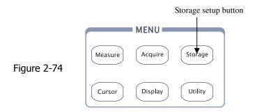
Press the Storage button to pop up the menu for the settings of the storage system. The waveforms and setups in both internal memory and external memory can be stored and recalled. The waveform file, setup file, bitmap and CSV file in external memory can be created and deleted. System supports English/Chinese key in.
