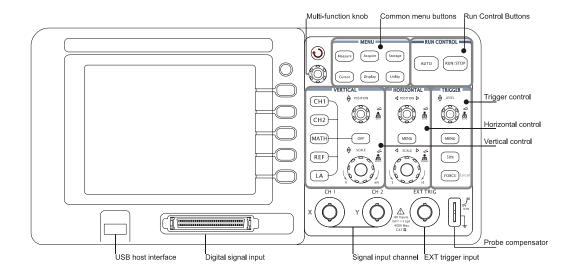
Figure 1-2 Front Panel Controls
