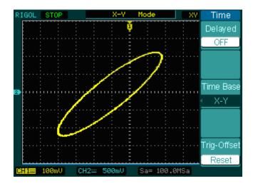
Figure 2-40: X-Y display format
