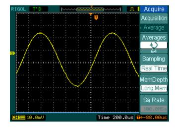
Figure 2-69: Display signal after average sampling
