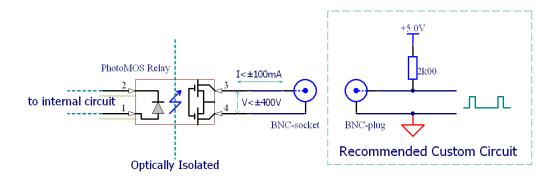
Figure 2-99 Schematic Diagram of Pass/Fail output
