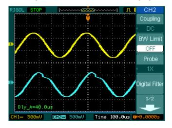
Figure 3-1: Delay of the signals
