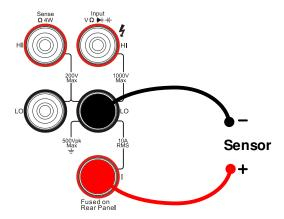
Figure 2-37 Current Sensor Connecting
