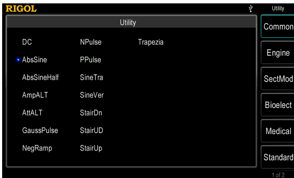
Figure 10-5 Waveform Defining Interface
