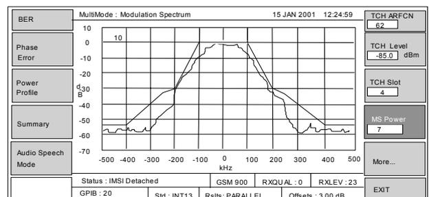
Real time displays for simple adjustments with superimposed limit mask
