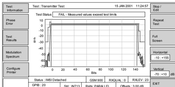
Graphic displays for fast recognition of failure modes
