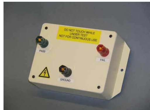
Figure 1: S14-01 Load Box
