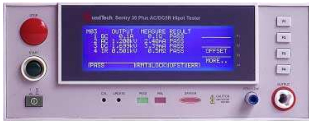
Figure 1-1: Sentry 30 Plus AC/DC/IR Hipot Tester
