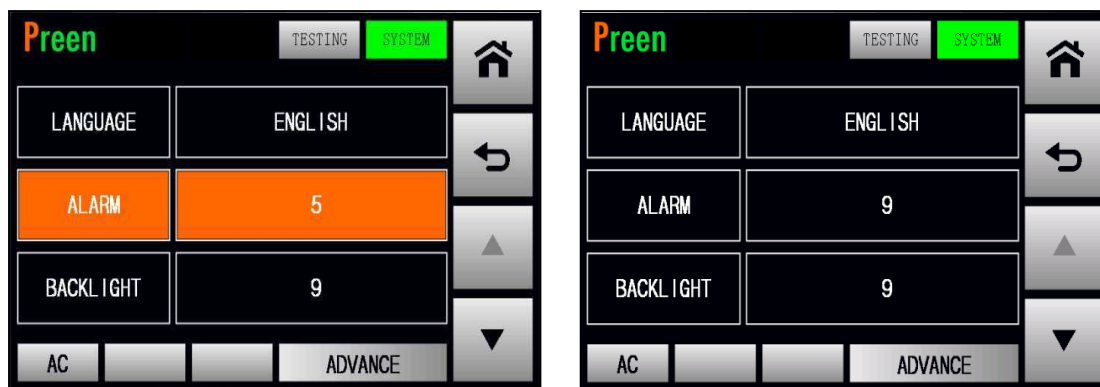
Figure 3-5-28 Set the alarm volume from 5 to 9.
