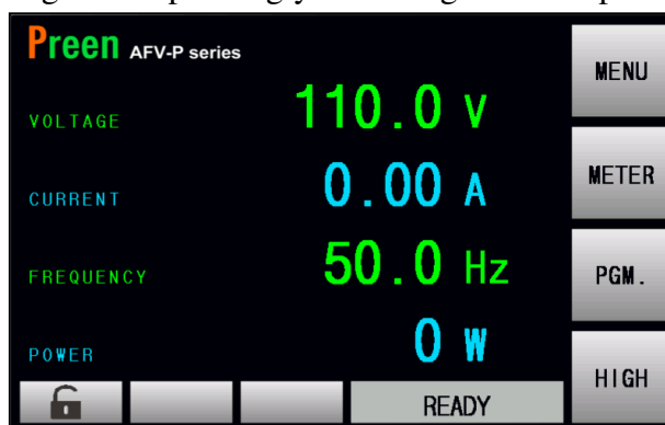
Figure 3-5-3 MAIN page when the output mode is AC.
