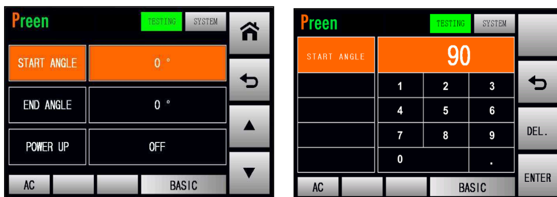
Figure 3-5-20 Set the start angle from 0° to 90° (BASIC mode).
