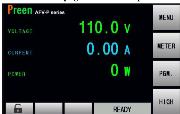
Figure 3-5-4 MAIN page when the output mode is DC.
