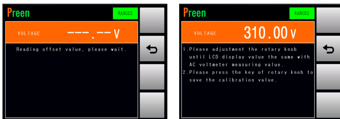
Figure 4-1-2 Enable the calibration of the HI-Range voltage 310V.
