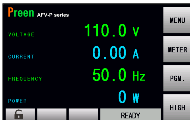
Figure 3-3-1 MAIN page when the product output is off.
