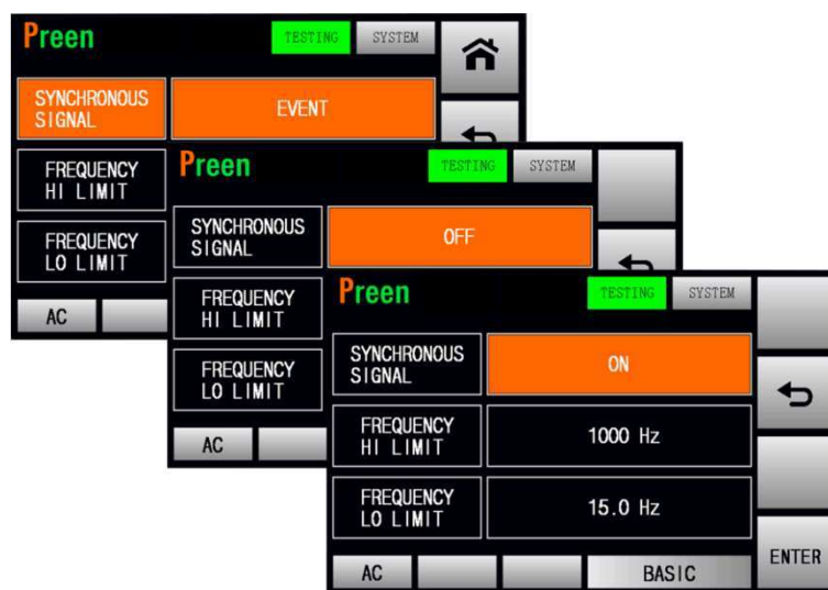
Figure 3-5-23 Three options of the synchronized signal (BASIC mode).
