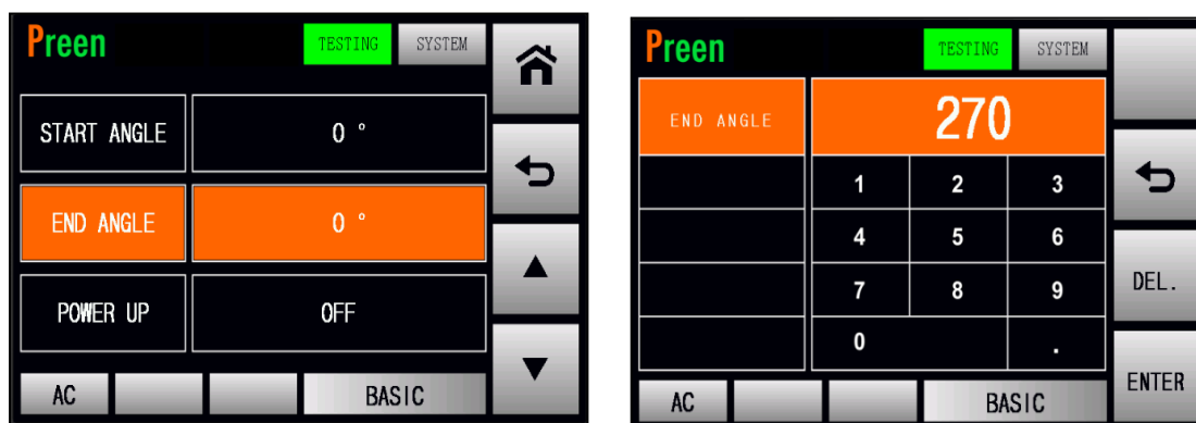
Figure 3-5-21 Set the end angle from 0° to 270° (BASIC mode).
