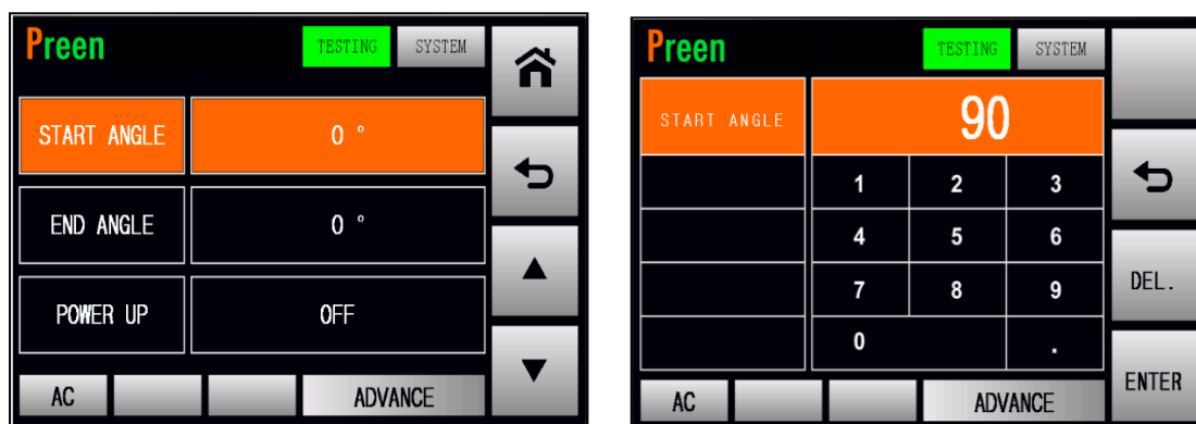
Figure 3-5-7 Set the start angle from 0^{\circ} to 90^{\circ} (ADVANCED mode).
