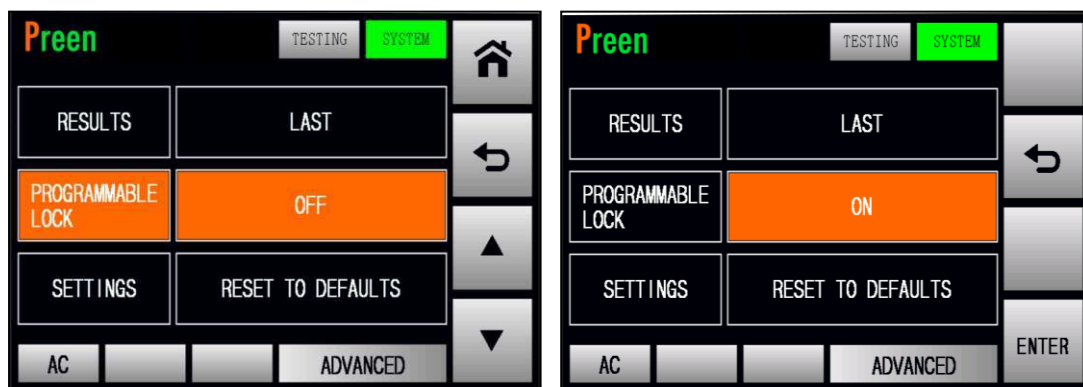
Figure 3-5-31 Unlock the PROGRAMMABLE feature.
