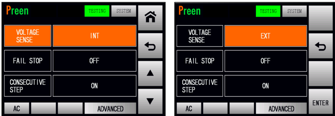
Figure 3-5-11 Set the voltmeter point from INT to EXT (ADVANCED mode).
