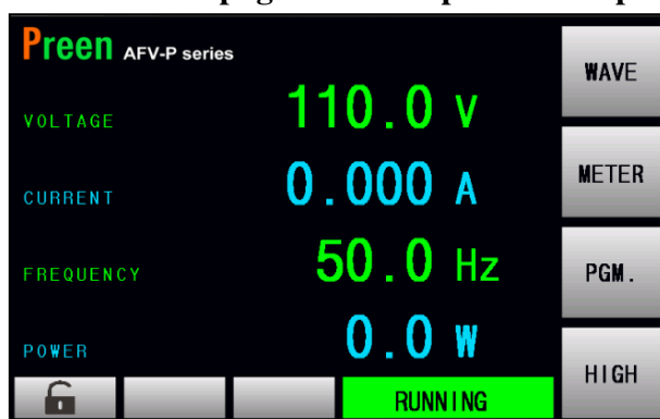
Figure 3-3-2 MAIN page when the product output is on.
