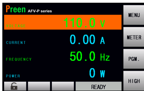
Figure 3-2-1 Press the desired item on the touch screen.
