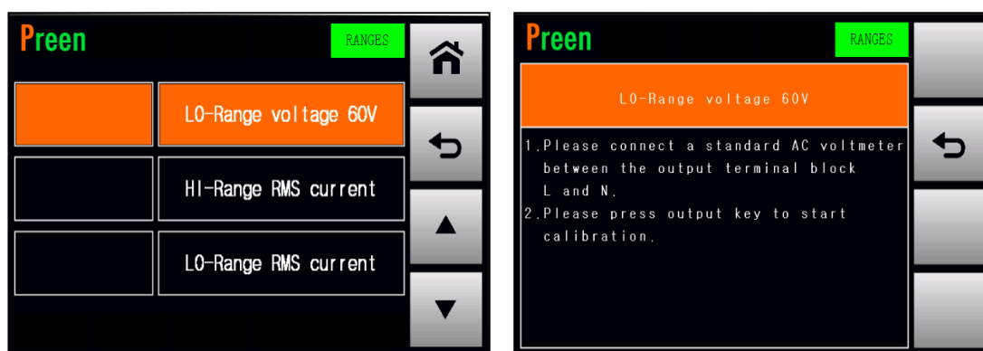
Figure 4-4-1 Enter into the page which calibrates the LO-Range voltage 60V.
