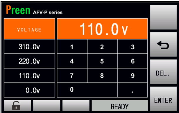
Figure 3-2-2 Virtual numeric and decimal keys.
