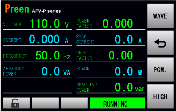
Figure 3-9-1 METER page when the product output is on.
