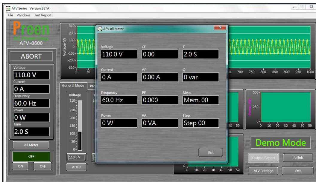
Figure 7-2-3 Show the measurement readings of the product output.
