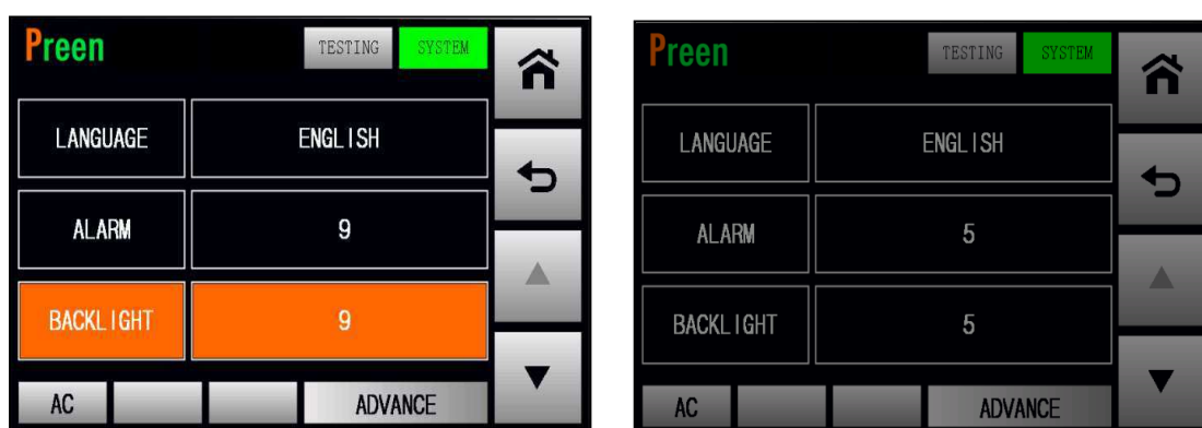
Figure 3-5-29 Set the backlight level from 9 to 5.
