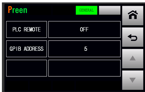
Figure 3-6-2 GENERAL subpage with the GPIB interface.
