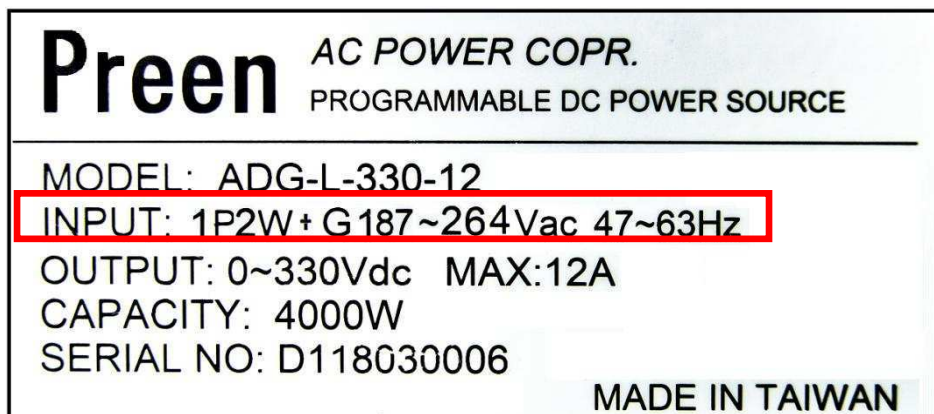
Figure2.2 Label sticker on the unit. (example of model ADG-L-330-12)
