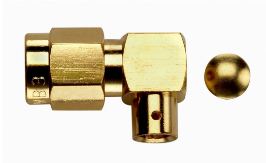
Model 72959 SMA PLUG R/A CRIMP, RG141, 174, 188, 316
