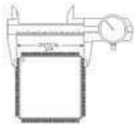
Measure Critical Dimension with calipers parallel to the plane of the PCB
