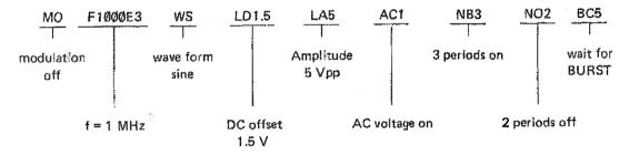
Note: Every string sent to the controller after 'IS?' begins with 'MO' (modulation off) to ensure safe acceptance of the string in every operation mode.
