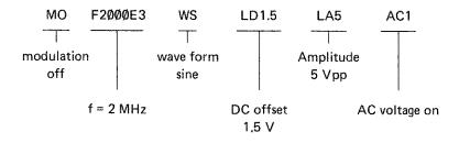
Note: Every string sent to the controller after 'IS?' begins with 'MO' (modulation off) to ensure safe acceptance of the string in every operation mode.
