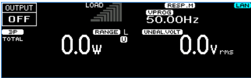
Single-phase display (example of U-phase display)
