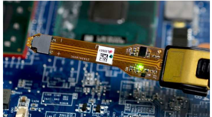
P77STFLXA solder down, flex-circuit accessory with an active buffer amplifier on its tip.
