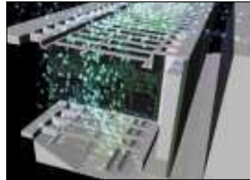
Figure 2. Computer modeling of the airflow aided the design of airflow deflectors and venting in the PXI-1006. This is a view of the card-cage from the right side of the PXI-1006.
