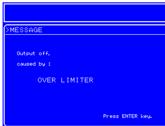
Figure 6-3. Warning Display Example
