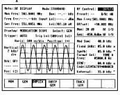
Full output level control from -130 dBm to 0 dBm over the entire range of the instrument is available from the RF I/O port (-130 dBm up to -50 dBm) and the generation port (-80 dBm to 0 dBm). Variable offsets from 0 to  $\pm$ 55 MHz in 5 kHz steps are keypad-selectable.
