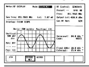
This display provides a clear graphic image of the audio baseband signal-selectable at either the vocoder input in generate mode or the vocoder output in monitor mode.
