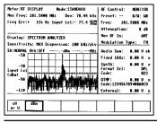
In addition to reading frequency error and modulation, a digital readout relative signal strength meter has been included. Sensitivity is specified to -100 dBm at the antenna port for FM signals and extends up to 125 watts at the RF I/O port. The CRT display will automatically convert to a terminating "watts" display as the level increases.
