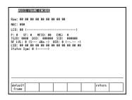
Conveniently accessed, dedicated test screens allow you to specify Link Control and Low Speed Data information contained within Voice Frames and to specify status symbol value. You can also set up from default values or operator specified input.
