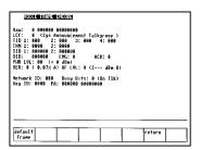
Conveniently accessed, dedicated test screens can be set up as a start-up default condition or a programmable test set-up. Dedicated ASTRO test screens are windowed with RF and Modulation control screens to simultaneously display test results along with their test conditions. While in ASTRO mode, standard diagnostic test screens can be easily accessed.
