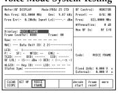
Project 25 compatible FDMA Digital C4FM modulation and either C4FM or CQPSK demodulation with vocoding and embedded data testing. Generate and monitor modes support actual functional voice testing. Within the voice mode, embedded data can be encoded and decoded for either subscriber or fixed site radio equipment.
