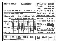
The System Analyzer includes the capability of encoding and decoding PRIVATE LINE (PL), DIGITAL PRIVATE LINE (DPL), and single tone sequences as well as multi-tone sequences including DTMF signals, 5/6 tone paging, Select V and up to 20 sequential tones. Decoding displays include tone frequencies and time durations of the individual tones. The unit can also encode tone remote signaling.
