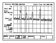
The built-in Spectrum Analyzer of the R-2660 will display a window of RF spectrum anywhere within the 400 kHz to 1 GHz operating range of the unit. The EXPAND softkey enlarges the display to fill the CRT and retains dispersion and center frequency control.
