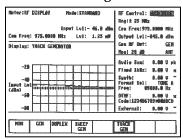
The combining of the capabilities of the sweep generator and the spectrum analyzer into a Tracking Generator function allows the user to view the performance characteristics of many RF filter devices. Display range is operator selectable from a 200 kHz window up to a 50 MHz window anywhere in the 400 kHz to 1 GHz spectrum.
