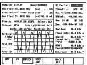
Full output level control from -130 dBm to 0 dBm over the entire range of the instrument is available from the RF I/O port (-130 dBm up to -50 dBm) and the generation port (-80 dBm to 0 dBm). Variable offsets from 0 to  $\pm 55$  MHz in 5 kHz steps are keypad selectable.
