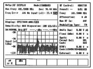
In addition to reading frequency error and modulation, a digital readout relative signal strength meter has been included. Sensitivity is specified to -100 dBm at the antenna port for FM signals and extends up to 125 watts at the RF I/O port. The CRT display will automatically convert to a terminating "watts" display as the level increases.
