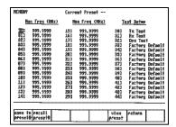
Channel Presets – The unit has 30 memory locations which can be used to store preset channel information. Channels can be easily selected individually or automatically scanned over a user defined range.
