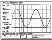
The oscilloscope has a 50 kHz bandwidth for audio waveform analysis. The display can be triggered over the full screen range to a fixed reference level. Triggering in both automatic and normal modes is provided for synchronizing the horizontal timebase to the vertical input signal. Internal or external inputs allow observation of both generated and monitored modulation signals. Softkeys provide for an enlarged full screen display.
