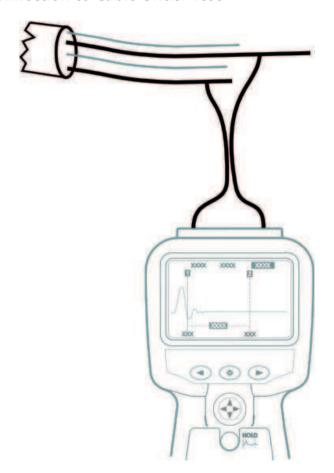
Connect the test lead to the cable under test. Connection may be made to a live power system with a voltage to earth (ground) less than 150 V with an installation (over voltage) category of I V or lower.
