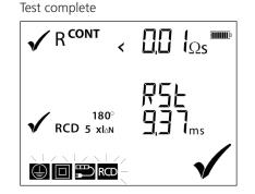
**Note**: The PAT150 defaults to 30 mA RCD. To change to 10 mA, hold the RCD button down for more than 2 seconds then release.
