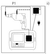
OR Insulation test @ 250 V
