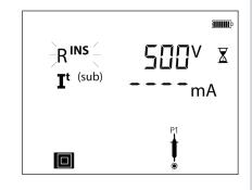
Repeat contact on all exposed conductive parts
