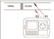
Connect both the P1 and P2 test leads to the circuit to be measured
