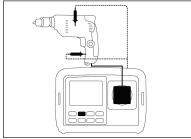
Connect the P1 test lead to different conductive points on the equipment under test during the measurement
