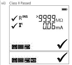
NOTE: High touch leakage measurement on faulty equipment can trip the supply RCD
