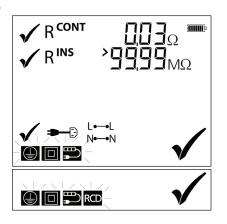
NOTE: For power cords longer than 5m the test can be re-run with a 1.0Ω pass limit by pressing the test button with 5 seconds of the continuity test failing – refer to page 13
