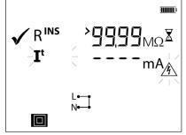
If the L to N short circuit symbol shows, user must check whether there is a true short circuit. Press Class II button to proceed but there is a risk of damage or tripping of protective devices.
