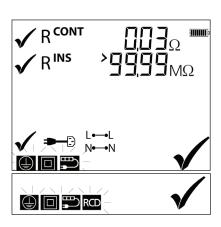
NOTE: Multiple earth continuity tests can be carried out by pressing the QT button during the continuity test, and pressing it again for each new continuity test. See Page 13
