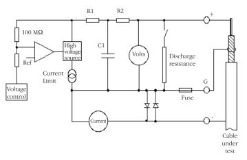
For 5 kV instruments C1 = 47 nF, R1 = 50 k $\Omega$ , R2 = 40 k $\Omega$
