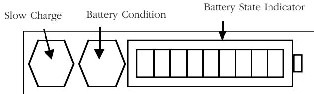
To find the amount of charge in your battery module, whether connected to your DLRO or separate, press the Battery Condition Button. The Battery State indicator will light between
