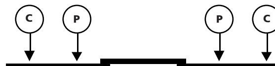
If using Duplex Handspikes ensure that the probe marked P is inside the C probes.
