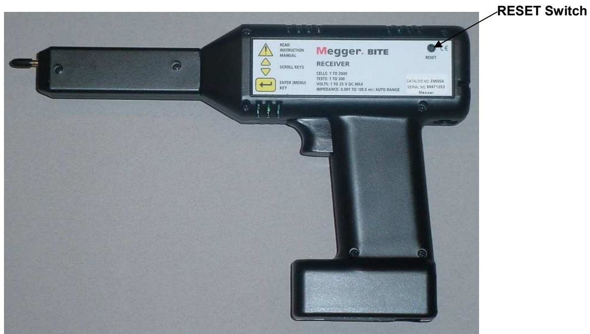
Figure 4-9: Receiver RESET switch
