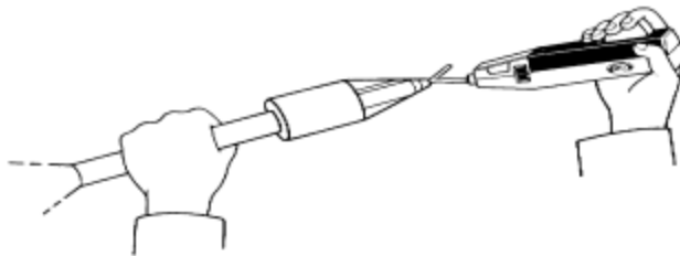
Figure 5: Using the Piezo Verifier to Check an LED Detector
