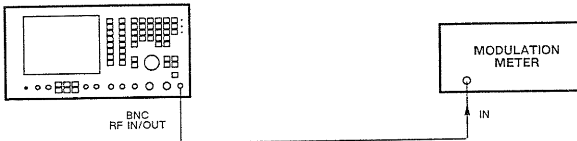
Fig. 6-23 Test equipment connections for RF generator AM depth and FM deviation
