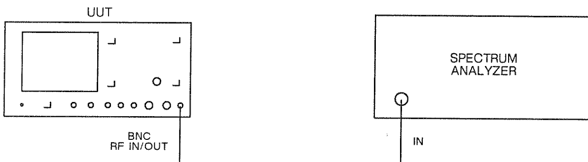
Fig. 5-26 Test equipment connections for RF generator harmonics, sub-harmonics and spurious signals
