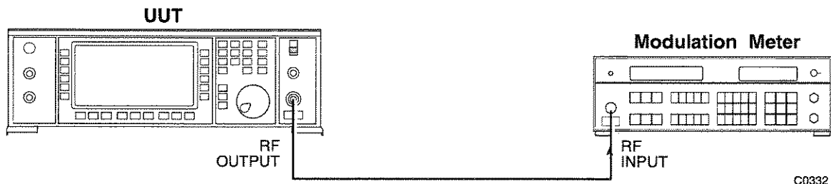
Fig. 5-1-9 Internal AM depth and distortion test set-up
