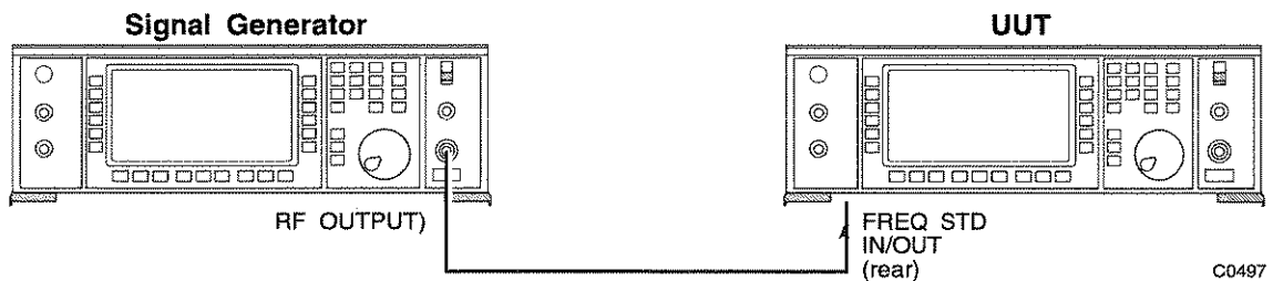
Fig. A-24 Frequency standard locking test set-up.
