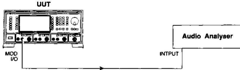
Fig. 7-15 Modulation oscillator distortion test set-up
